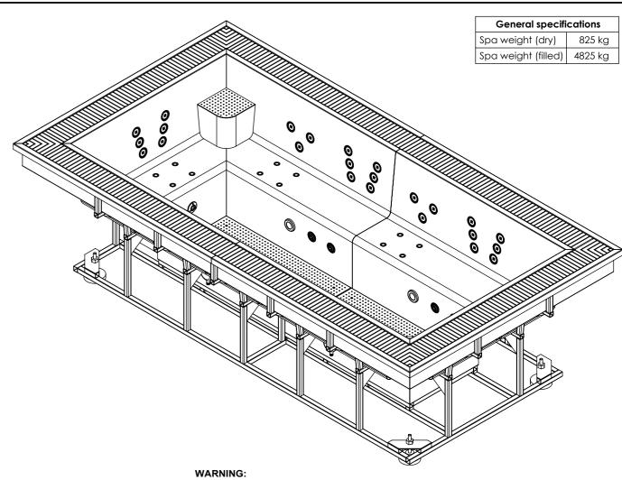
It's essential to keep a minimum clearance access of 700mm all around. Minimum depth of spa hole 920 mm.
